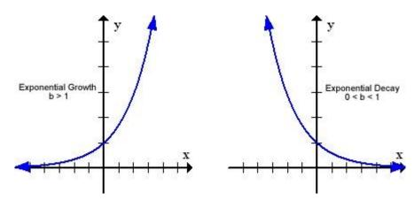
Looking at the graphs shown above, we can see that no horizontal line can be drawn that would intersect the graph of the exponential functions at more than one point. This means that exponential functions are one-toone functions and one-to-one functions must have an inverse. So, let's try and find the inverse of an exponential function,  $f(x) = b^x$ . Here are the steps for finding the inverse function.
